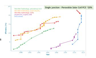
Perovskite solar cell technology is the most rapidly developed solar technology ever – from 3% (2009) to 20% (2015). Promising prospect of reaching PCE >25 % in single junction and PCE >30% in tandem junction.
